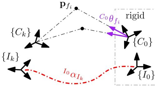
Fig. 2: Frame of references used in the problem. Two features observed from both the  $\{C_k\}$  and  $\{C_0\}$  frame are shown. The transformation from the  $\{I_k\}$  and  $\{I_0\}$  is found through IMU integration. The bearing  ${}^{C_0}\theta_{f_i}$  is used along with the scale-less depth to recover the scale  $a$  and shift  $b$ .
