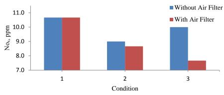
Figure 5. Graph of NO<sub>X</sub> composition at constant engine speed
