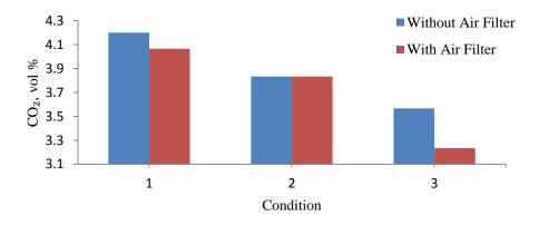
Figure 4. Graph of CO<sub>2</sub> composition at constant engine speed
