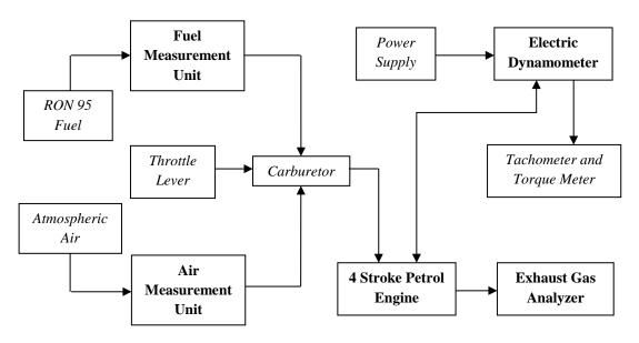
Figure 1. Overall experiment instrument layout.
