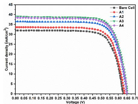
Fig. 8. Photovoltaic performance of the spinel  $MnFe_2O_4$  coated solar cell compared with the bare cell under closed atmospheric conditions.
