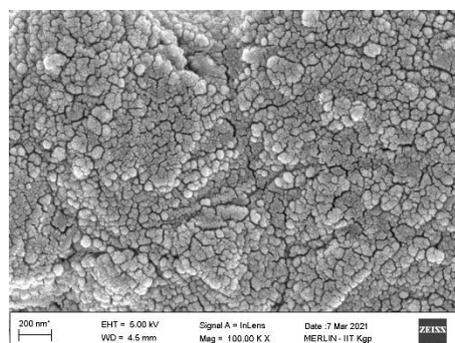
Fig. 5. a) FESEM image of  $\text{MnFe}_2\text{O}_4$  Coated A3 Layer on Silicon solar cell.
