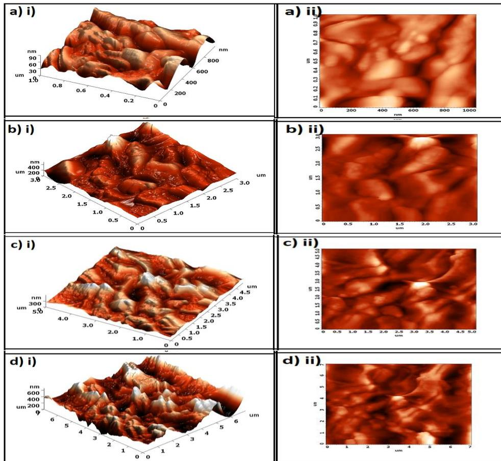
Fig. 4. AFM images of a) single layer coating b) Double layer coating c) Three layer coating d) Four layer Coating.
