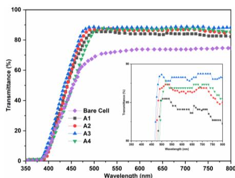
Fig. 6. Optical Transmittance of  $MnFe_2O_4$  solar cells.
