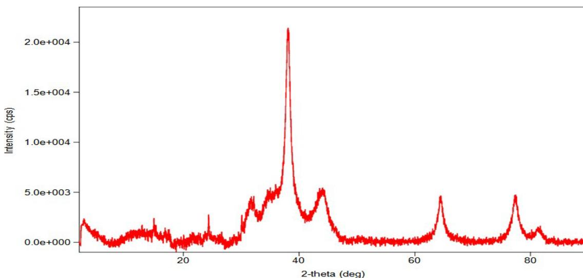
Fig. 5. XRD spectra of biosynthesized silver sulfide Nano particles.
