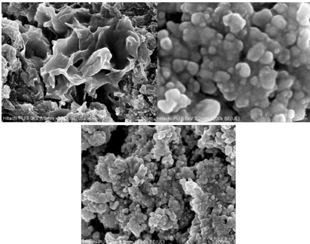
Fig. 6. SEM spectra of biosynthesized  $\text{Ag}_2\text{S}$  Nano particles
