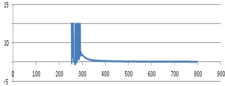
Fig. 2. UV spectra green synthesized silver sulfide NP'S
