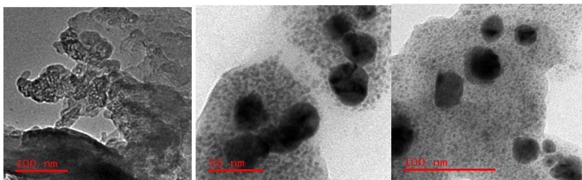
Fig. 8. TEM Images of Biosynthesized silver sulfide nanoparticles.
