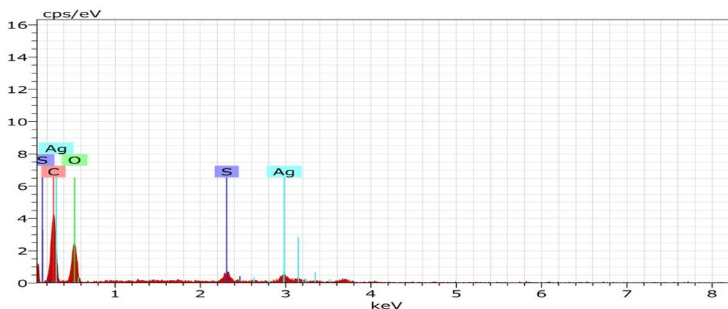
Fig. 7. EDX spectra of biosynthesized  $Ag_2S$  Nano particles.
