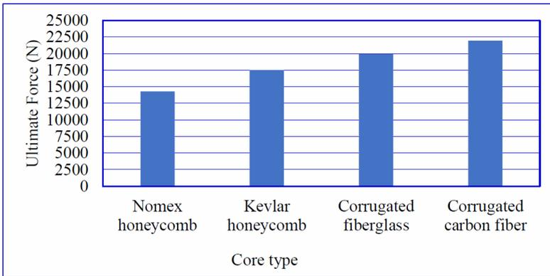
**Figure 6** Amount of energy absorbed by sandwich structure members with carbon facings and different core type (see online version for colours)
