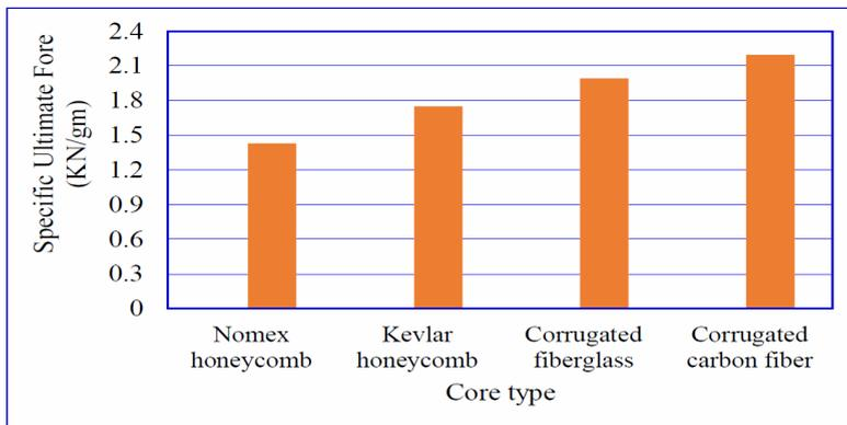
**Figure 9** Specific energy to weight ratio of sandwich structure members with carbon facings and different core type (see online version for colours)
