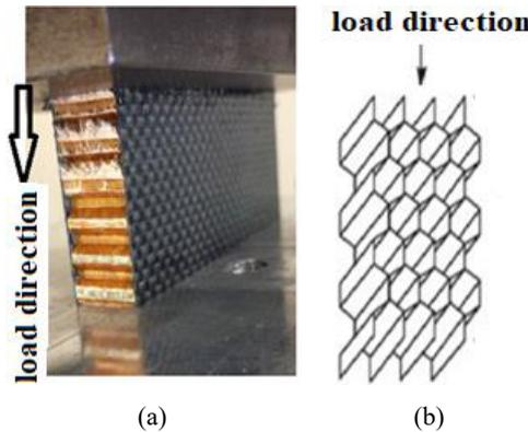
**Figure 2** Samples positioning during testing and the load direction, (a) a sample with a honeycomb core (b) load direction with respect to the hexagonal cell (c) a sample with a corrugated core (d) load direction with respect to the corrugation (continued) (see online version for colours)
