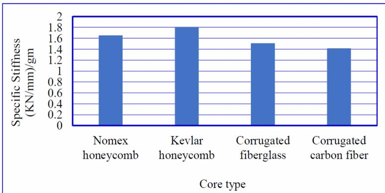
**Figure 8** Specific ultimate compression force to weight ratio of sandwich structure members with carbon facings and different core type (see online version for colours)
