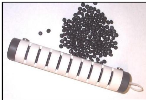
*Fig. 1 - Bio-Trap<sup>®</sup> sampler from Microbial Insights, Inc.*
