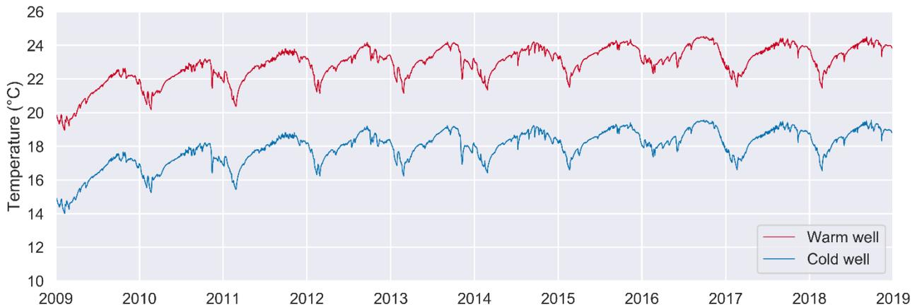
Fig. 1 - Simulated groundwater temperature evolution at the ATEs wells (warm and cold wells) over the 10 years simulation period.
