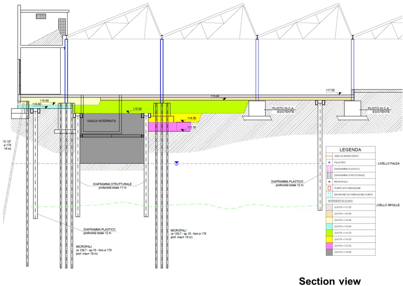
Fig. 1 - Section view of the realized physical containment
