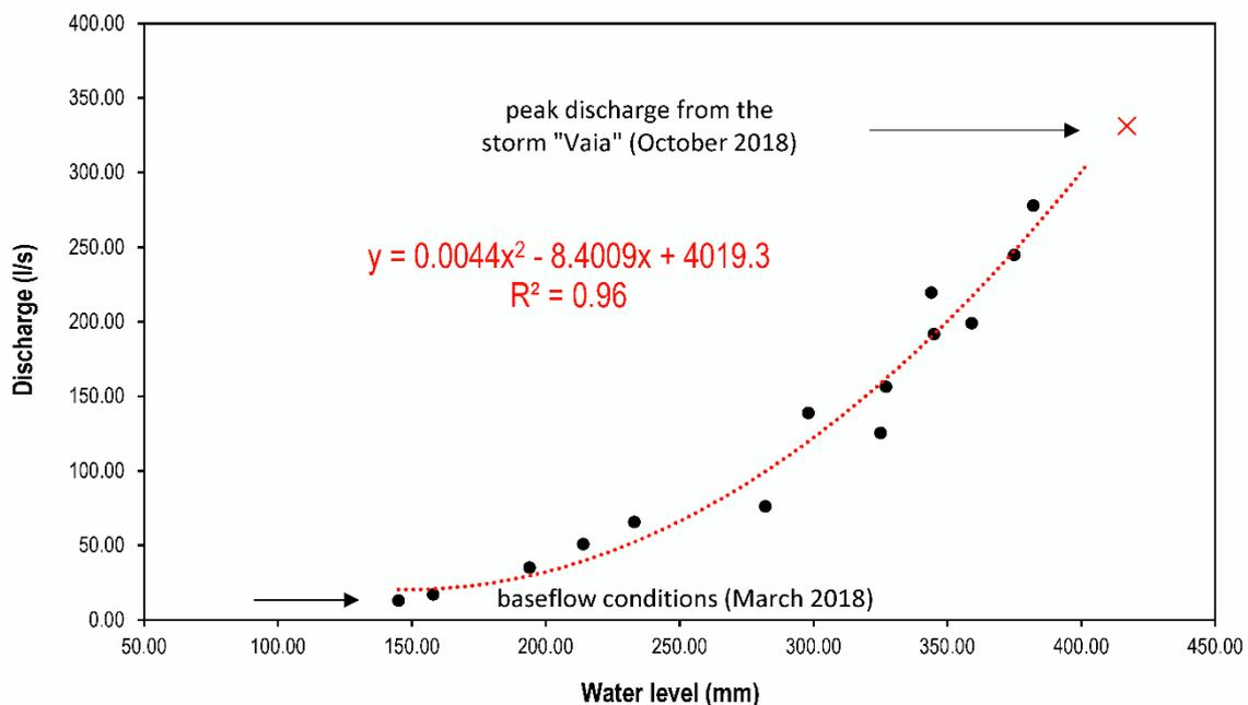
Fig.1 - Stage-discharge rating curve of the Pradidali karst spring. Water level-discharge pair for the storm Vaia is also represented in the figure. The discharge was extrapolated from the fitting function.
