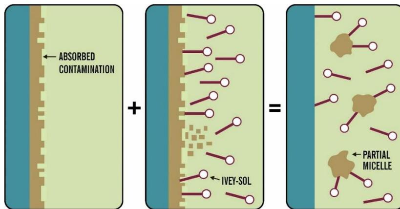
*Fig. 1 - Operating principle of Ivey-sol<sup>®</sup> surfactants*
