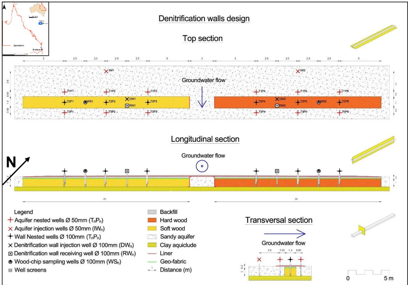
Fig. 1 - The two twin denitrification walls installed on the pineapple farm located 70 Km North of Brisbane.
