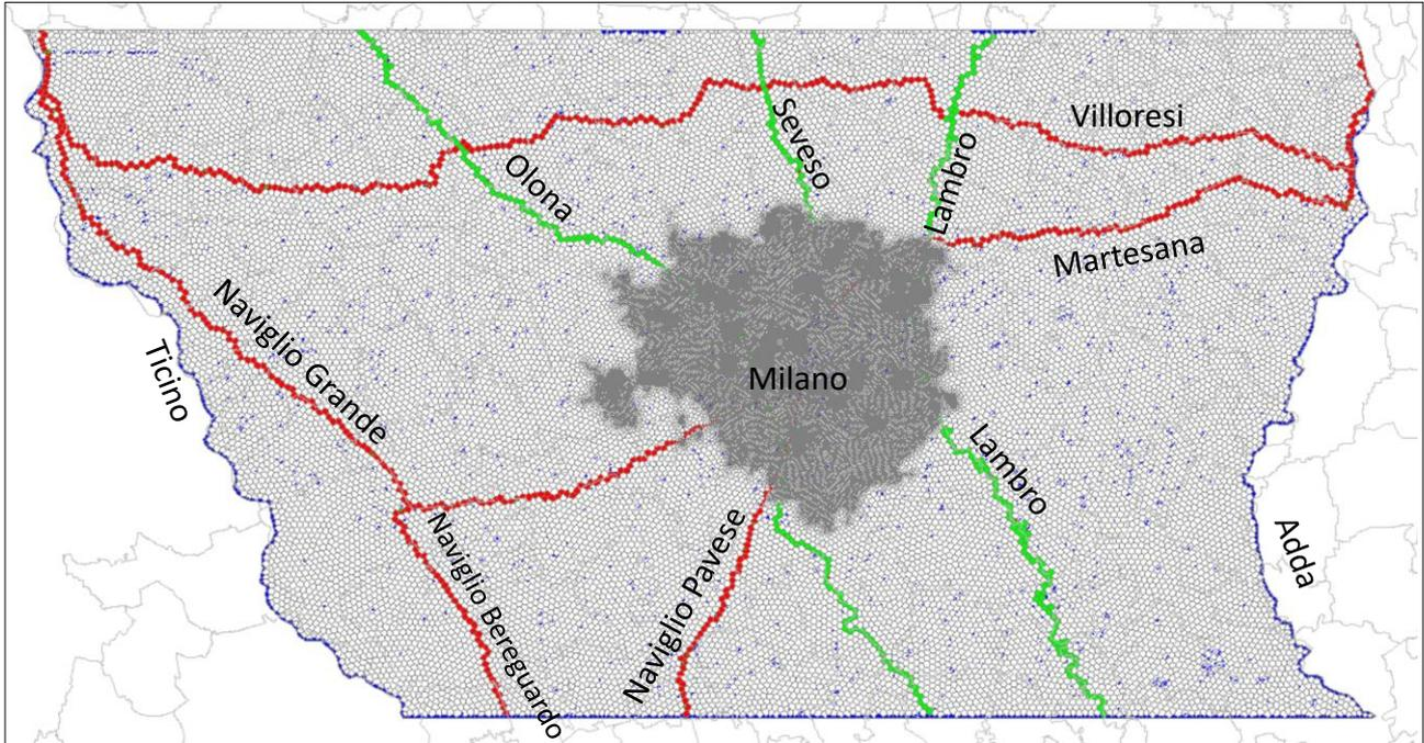
Fig. 1 - Numerical flow model implemented using a Voronoi mesh. Rivers inside the model are represented in green (in blue the ones at the boundary: Ticino and Adda), channels are shown in red while blue points are wells.
