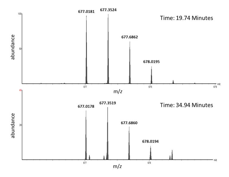
**S3 Fig**. HR-MS spectra from the data set used to generate the plot in Fig 3. Top, spectrum from 19.74 minutes (beginning of the plot). Bottom, spectrum from 34.94 minutes (end of the plot). The similarities between the two are obvious. All intervening spectra were similar.
