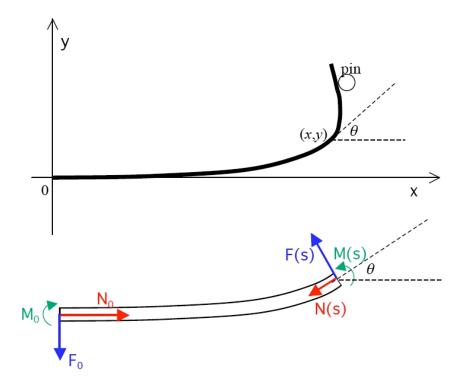
Figure A1. Elastic beam. Top: coordinates used in the calculation.  $\theta$  is the angle between the beam tangent vector and the *x*-axis. Bottom: A segment of the beam, between the origin and *s*, showing the forces and moments applied to the ends. Red: normal forces. Blue: shear forces. Green: bending moments. Note that the bending moment at *s* is defined to be positive if it produces an upward curvature.
