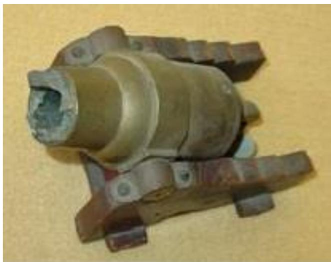
**Fig. 56.** Spanish gun failure due to compressed powder
