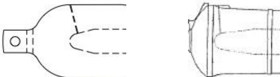
**Fig. 32.** Breech and chamber of Dahlgren 9in SB
