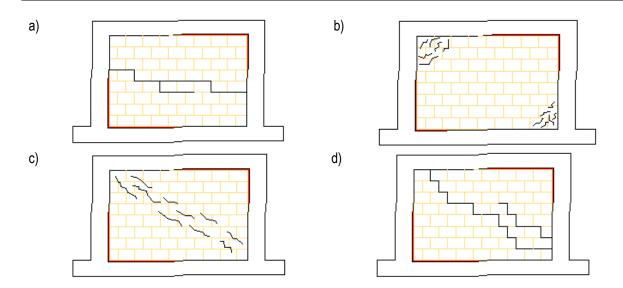
Figure 1.Equivalent strut, showing the modes of failure for the infill:
