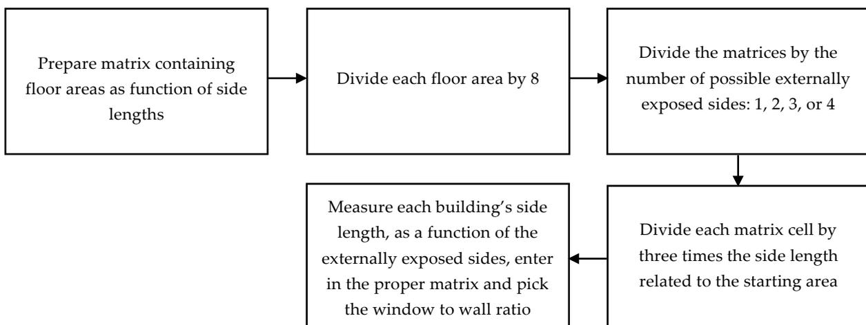
Fig. 1 – Window to wall ratio evaluation flowchart
