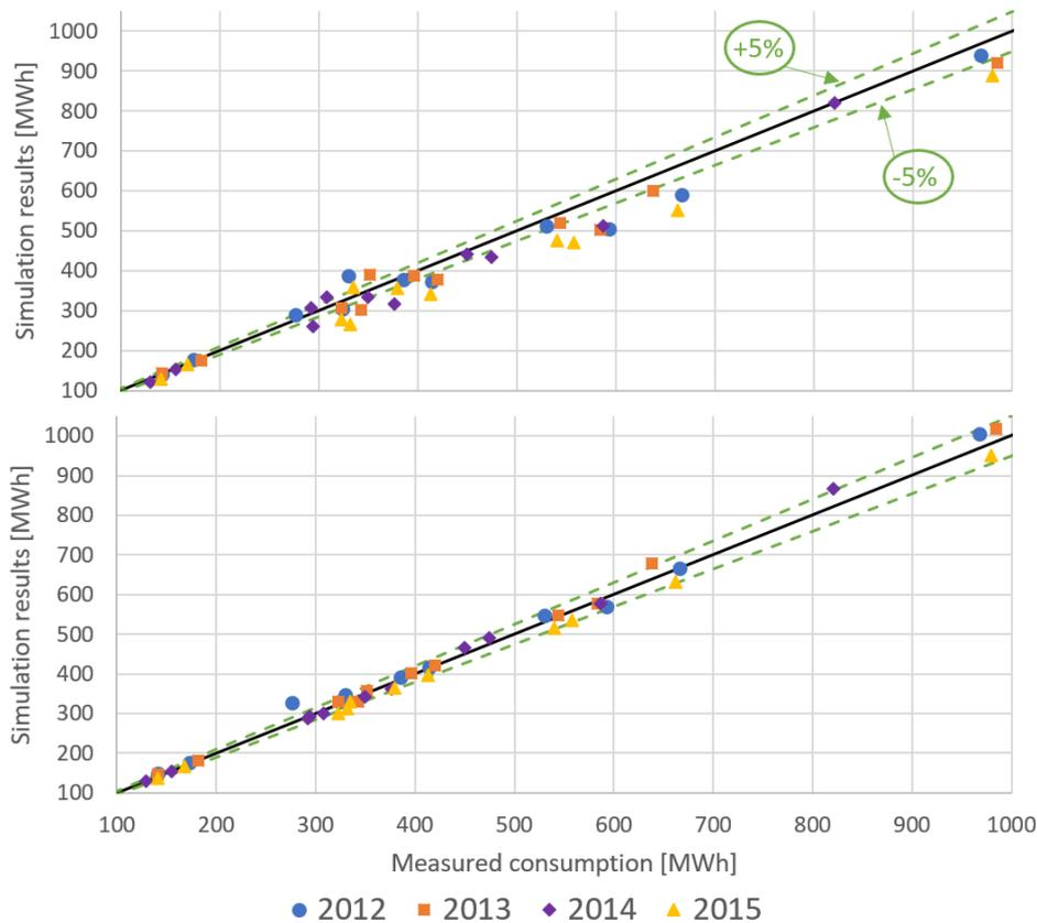
Fig. 5 – Heating demand results prior and after calibration
