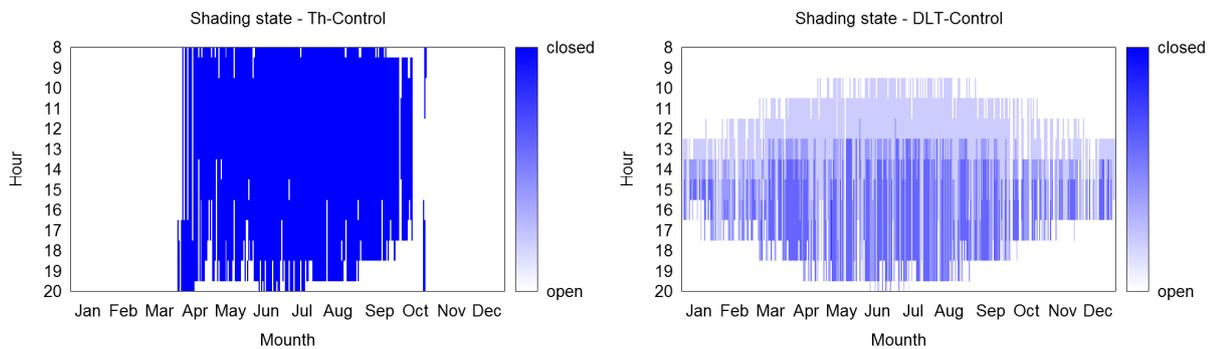
Fig. 16 – Hourly shading schedule. The several states available to the *DLT-Control* allow for a better control of the incident daylight, hence providing optimum illuminances in the range from 300 to 3000 lux.
