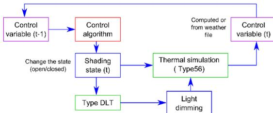
Fig. 11 – *Th-Control* algorithm
