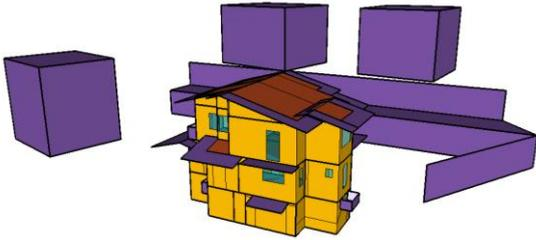
Figure 3 – Complete model for building envelope (Trnsys3D)
