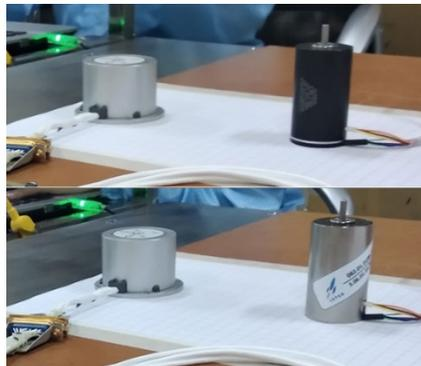
Fig. 5 Magnetic field measurements of unshielded motor (above) and shielded motor (bottom)
