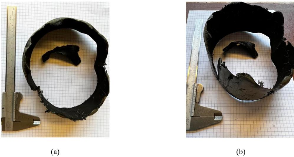
Figure 14: 5MgB<sub>p</sub> grain; paraffin +5%MgB<sub>2</sub> solid fuel after test 2, burning time of 5.1 seconds
