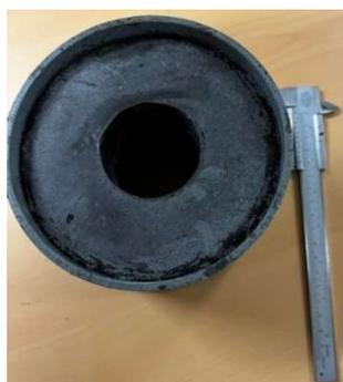
Figure 6: ULB-HRM paraffin solid fuel grain doped with  $\text{MgB}_2$
