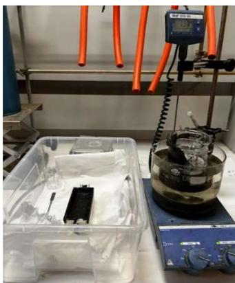
Figure 5: MOUETTE fuel grain during the manufacturing process (right) and sample in the mould (left)
