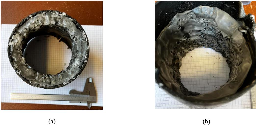
Figure 13: Pure paraffin solid fuel after test 1, burning time of 5.1 seconds
