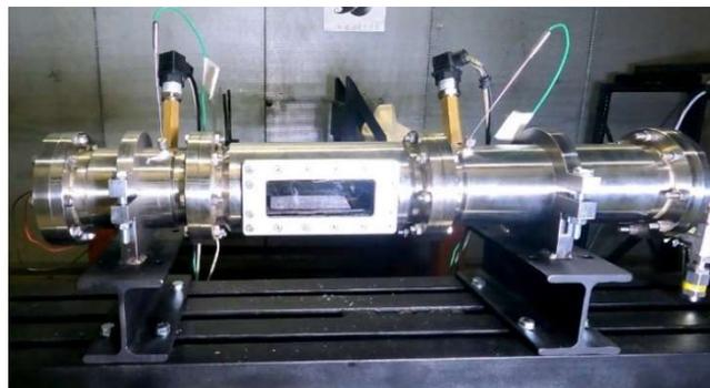
Figure 3: MOUETTE slab-burner with a paraffin grain doped with 5%  $MgB_2$
