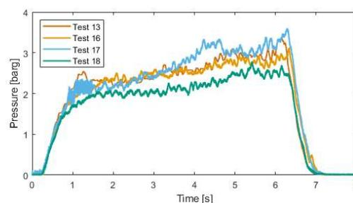
Figure 8: Tests #13 and #16 (10MgBp); #17 and #18 (5MgBp) – Paraffin + additives
