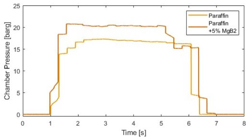
Figure 15: Chamber pressure for the test 1 and test 2
