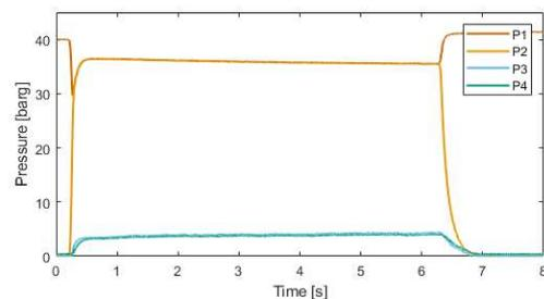
Figure 9: Feed-system pressure budget, test 8
