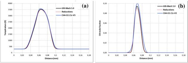
Figure 14 : Axial temperature profiles (a) and OH molar fraction profile (b) through the counter-diffusion flame for different kinetic schemes
