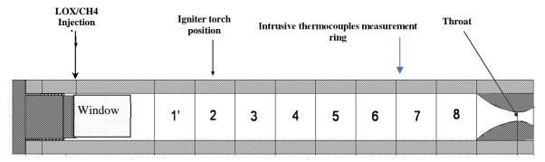
Figure 1: BHP combustion chamber set-up schematic
