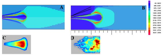
Figure 15. Calculated temperature map (A) G2 operating point (B) T1 operating point (2D calculations) – average OH\* emission for G2 operating point (C)\* instantaneous OH\* emission for T1 operating point (D)\* (extracted from [2]).
