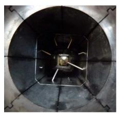
Figure 7 - Intrusive thermocouples positions in BHP chamber 7th module – Visualization from downstream
