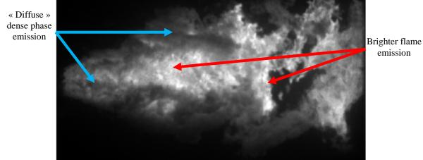
Figure 9. Evidence of "diffuse" dense phase emission around brighter flame emission – Instantaneous OH\* emission image - TL operating point
