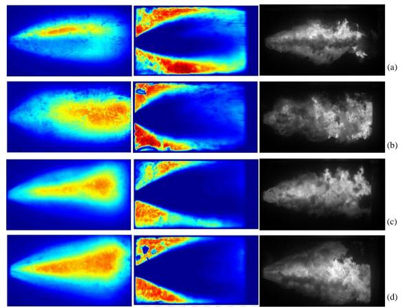
Figure 8. Time-averaged OH\* emission (left), time-averaged shadowgraphs (center) and instantaneous OH\* emission (right) for operating points LH (a), LL (b), TH (c), and TL (d).
