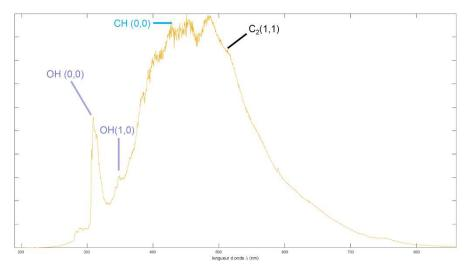
Figure 5. Emission spectrum of the LOX/CH4 flame at LH operating point
