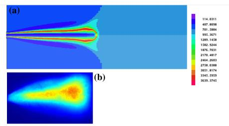
Figure 18. Temperature map for TH operating point – 2D calculation (a) – averaged OH\* emission (b)
