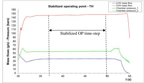
Figure 3 – Typical temporal evolution of mass flows and chamber pressure over stabilized operating point (TH) time step
