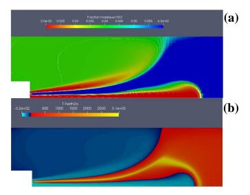
Figure 16. Calculated H<sub>2</sub>O mass fraction (a) map of delta-temperature to H2O local saturation temperature (b) in the near injection region for T1 operating point (2D calculations)
