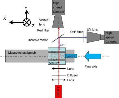
Figure 6: Imaging setup arrangement (top view) with shadowgraphy and chemiluminescence visualizations
