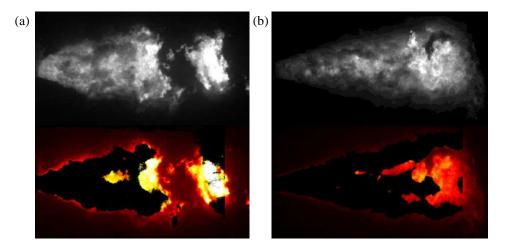
Figure 11. Instantaneous OH\* emission in grey levels scale (up) and superposed instantaneous OH\* emission and binarized shadowgraphs (down) for recessed injector (a) and non-recessed injector (b) @ TH operating point.
