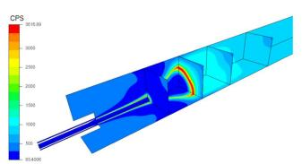
Figure 17. Calculated temperature map for T1 operating point (3D calculation)
