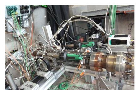
Figure 4. Optical diagnostics implemented on MASCOTTE test bench – Simultaneous high-speed OH\* chemiluminescence and shadowgraphy
