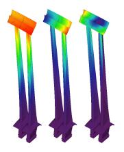
Figure 3: Modal shapes for welded in pairs configuration. Modes 1 to 3 from left to right.
