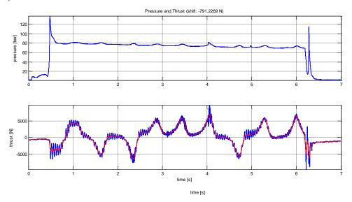
Figure 11a-b: ACS trial combustion chamber pressure (a) and Thrust (b)
