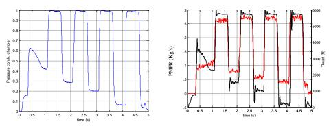
Figure 6a-b: GRM-02 Combustion chamber pressure (a), PMFR and Thrust (b)
