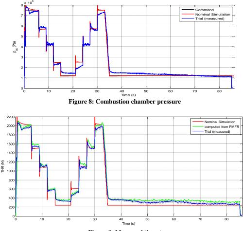
**Figure 9: Measured thrust**
