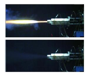
Figure 7: High speed photos during ignition and after ignition end
