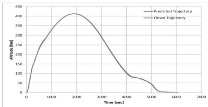
Figure 9 – Flown vs predicted trajectory of IXV
