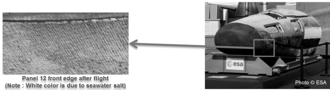
Figure 11 –Panel 12 front edge after flight
