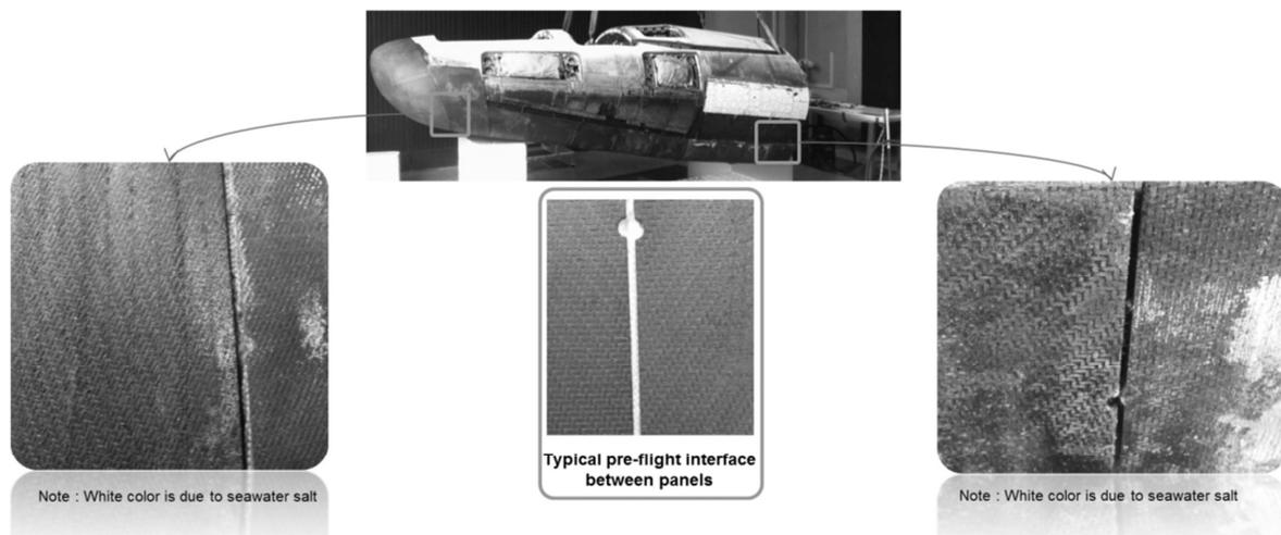
Figure 5 – Visual inspection of TPS after re-entry
