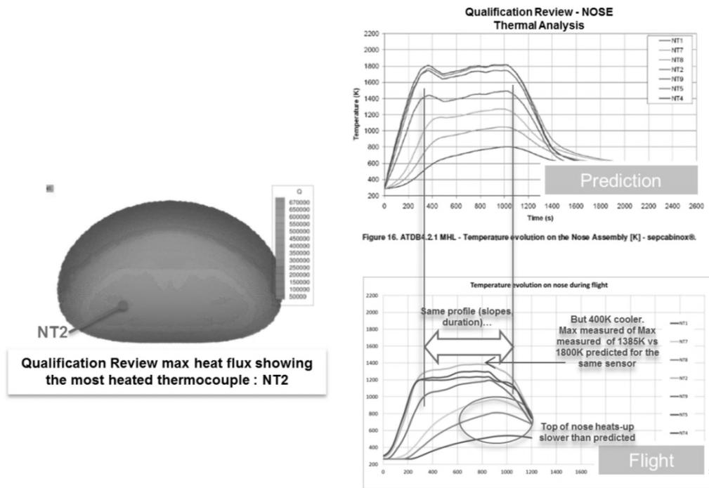
Figure 8 – comparison between predictions and measures for panel 27
