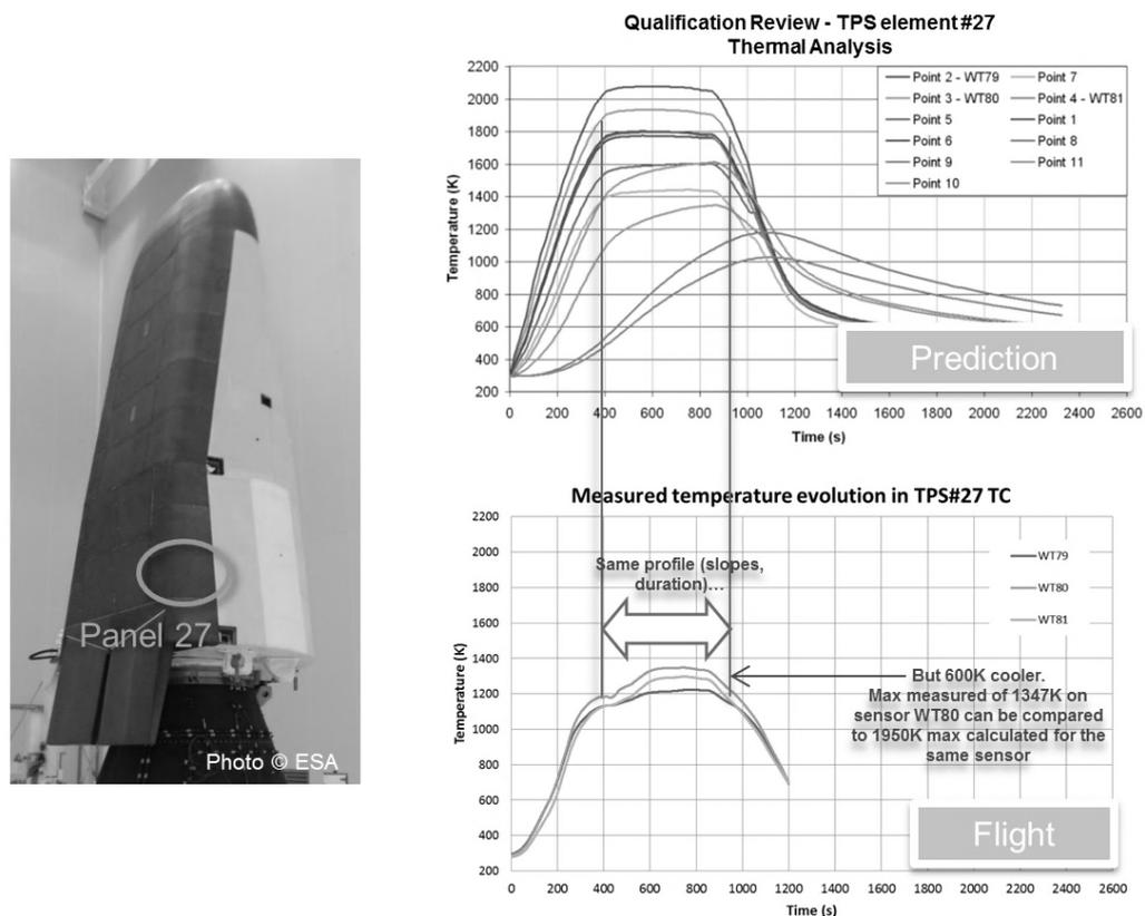
Figure 7 – comparison between predictions and measures for panel 27
