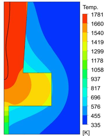
Fig. 5. Temperature field after solidification of the casting at  $t = 488$  s, II variant.
