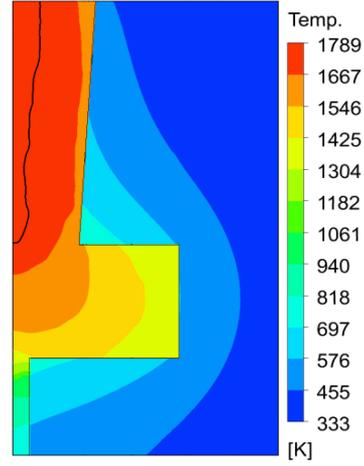
Fig. 4. Temperature field after solidification of the casting at  $t = 562$  s, I variant.
