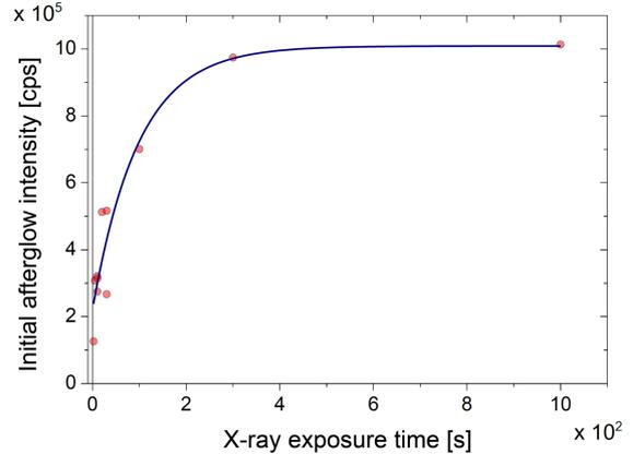
Fig. 4. Dependence of the initial afterglow intensity upon the X-ray exposure time. The solid line represents an approximation of experimental points by the function.
