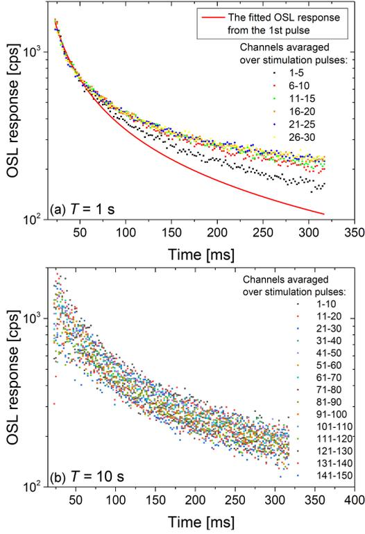
Fig. 5. The OSL response of the YAP:Mn crystal on the blue light (470 nm) stimulation by pulses of 10 ms duration registered as photon-counting in the channels of 2 ms duration at pulses repetition period 1 s (a) and 9 s (b).
