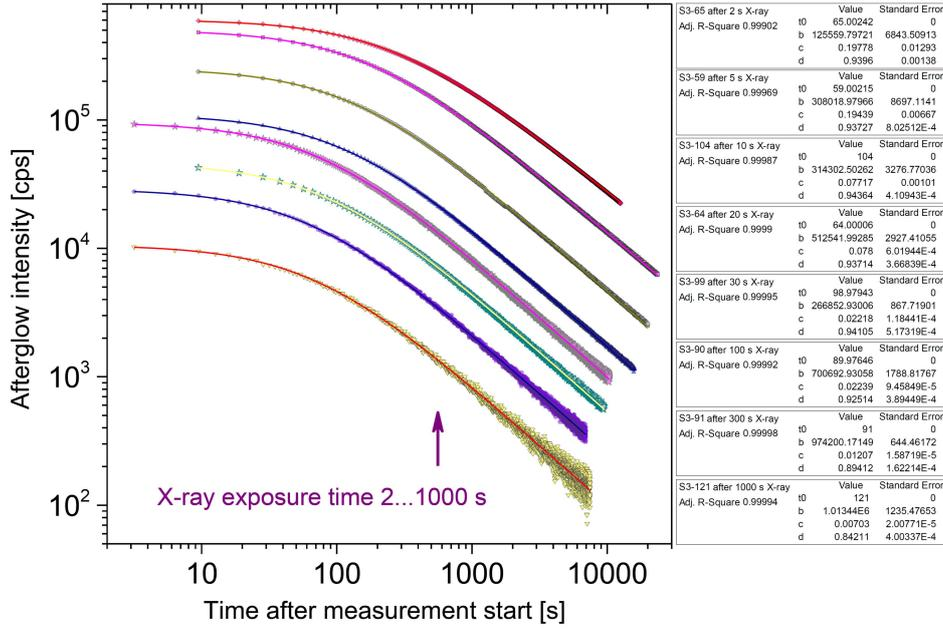
Fig. 3. The X-ray produced afterglow (points) of YAP:Mn crystal after different irradiation times and the corresponding fitted dependencies (solid line) in the form of (2). The inset represents the parameters of fitted functions. The last number in the sample notation (S3-##) shows the time delay  $\Delta t$  [s] from the end of irradiation till start of measurement. Other notations represent the values in (2):  $t_0 - \Delta t$ ,  $b - I(0)$ ,  $c - w$ ,  $d - \alpha$ .
