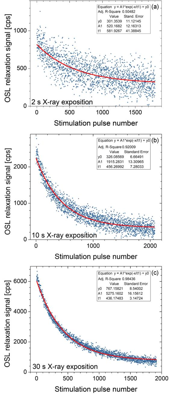
Fig. 6. The dependence of the rapid component of the YAP:Mn OSL response upon stimulation pulse number with repetition period 1 s for the X-ray irradiation during 2 s (a), 10 s (b) and 30 s (c). Experimental data are represented by points and their approximations by the function (3) are drawn by solid line. The insets demonstrate parameters of fitted functions.
