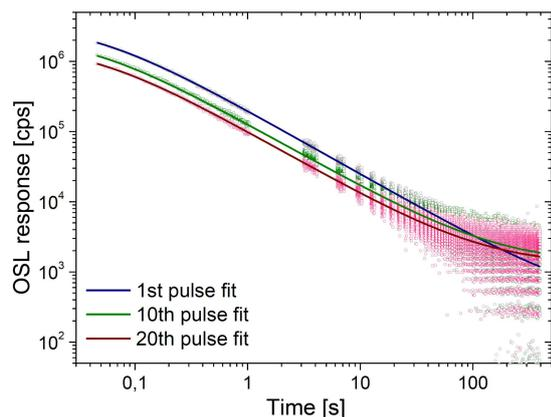
Fig. 1. The YAP:Mn OSL decay curves (points) recorded after the 1st (violet), 10th (olive) and 20th (purple) sequential pulses of 100 ms duration of blue (470 nm) light stimulation together with their fits (solid lines) by mean of function (1) with some background from [9]. The repetition period of stimulation pulses was equal to 420 s.
