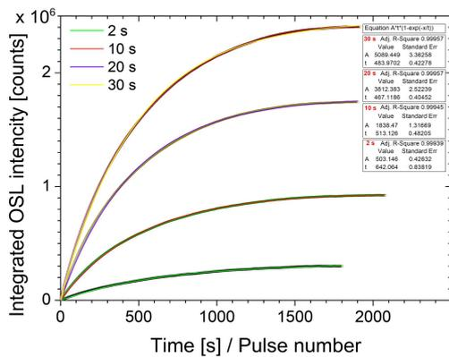
Fig. 7. The integrated rapid component of the OSL response vs pulse number for different X-ray exposure of YAP:Mn crystal. Experimental data are represented by points and their approximations by the function (4) are drawn by solid line. The insets demonstrate parameters of fitted functions.
