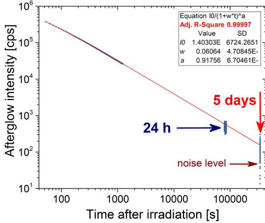
Fig. 2. The kinetics of green afterglow (points) of YAP:Mn crystal induced by the X-ray irradiation during 30 s (absorbed dose about 0.9 Gy) and its fitting (solid line) by the function (1). The inset represents the parameters of fitted function.
