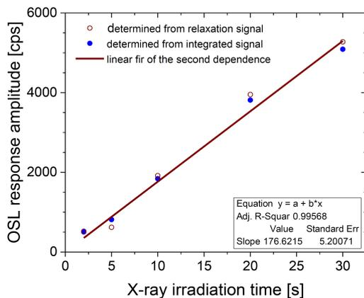
Fig. 8. The dose dependencies of the YAP:Mn crystal OSL response amplitude and the amplitude of the integrated OSL response upon the X-ray exposure time in the range 2–30 s, and linear fit of the last.
