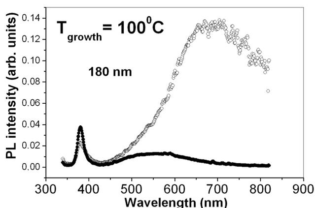
Fig. 3. Room temperature photoluminescence spectra of ZnO films grown at 100 °C before (open circles) and after optimization (solid circles).
