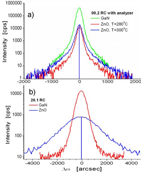
Fig. 2. The comparison of the rocking curve of the monocrystalline ZnO films grown at 280 °C (S396) (a) with a rocking curve of a GaN/ $\text{Al}_2\text{O}_3$  substrate (b).
