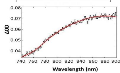
**Step 3:** Modified Beer-Lambert's law that associates measured  $\Delta OD$  values over  $n$  wavelengths with changes of concentrations in  $\Delta[HbO]$ ,  $\Delta[HHb]$  and  $\Delta[CCO]$ .
