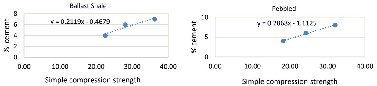
Figure 4 (a) Simple Compression Strength vs % Cement; Ballast Shale; (b) Simple Compression Strength vs % Cement; Pebbled
