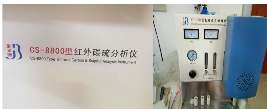
Figure 1s: CS-8800 type infrared Carbon and Sulphur analysis instrument
