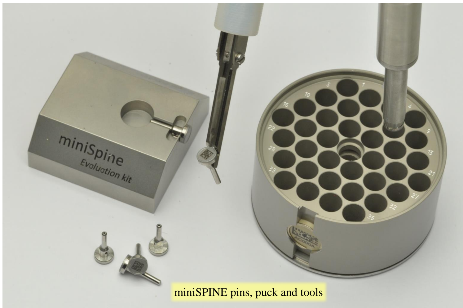
Figure S 3: miniSPINE sample holders, puck and manual handling tools (picture)
