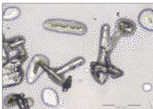
b) T = 140.0 °C (melting process starts)
