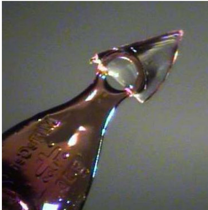
Figure S1. Mounted crystal of RuPhos.
