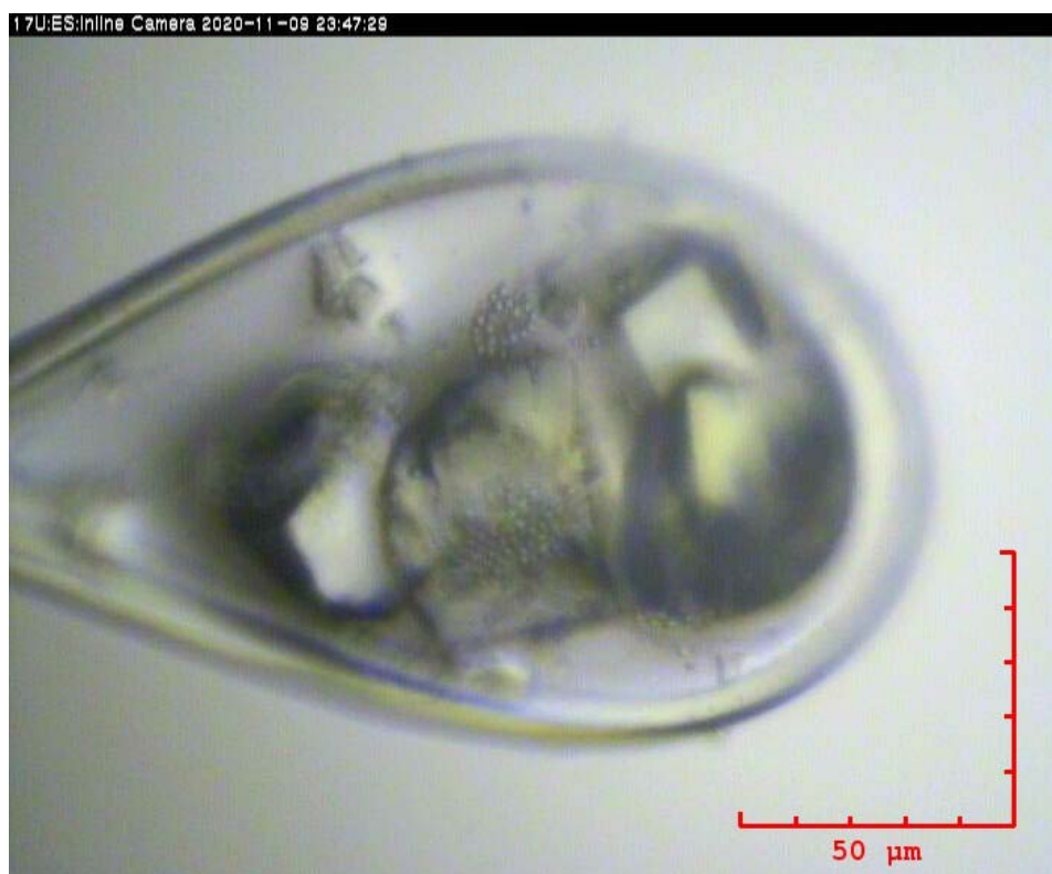
Figure S1 A view of four lysozyme crystals placed in a cryo-loop, taken by an on-axis camera.
