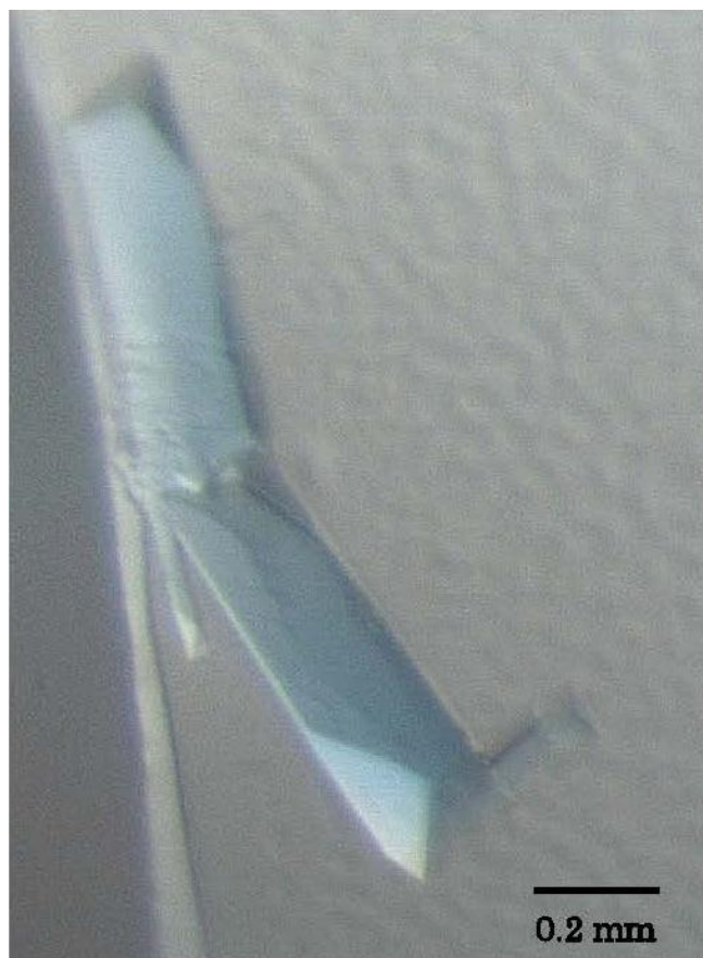
Figure S3 CueO-d crystal. Scale bar corresponds to 0.2 mm. The dimensions of the crystal are 0.5 x 0.2 x 0.2 mm 3 .
