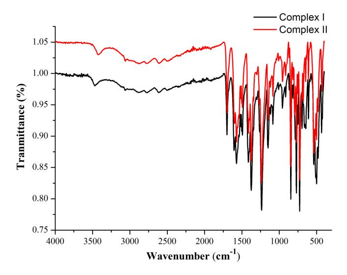
Fig. S1. The IR spectra for **I** and **II** recorded from a KBr pellet in the range 4000-400 cm<sup>-1</sup> on a Bruker ALPHA spectrometer.
