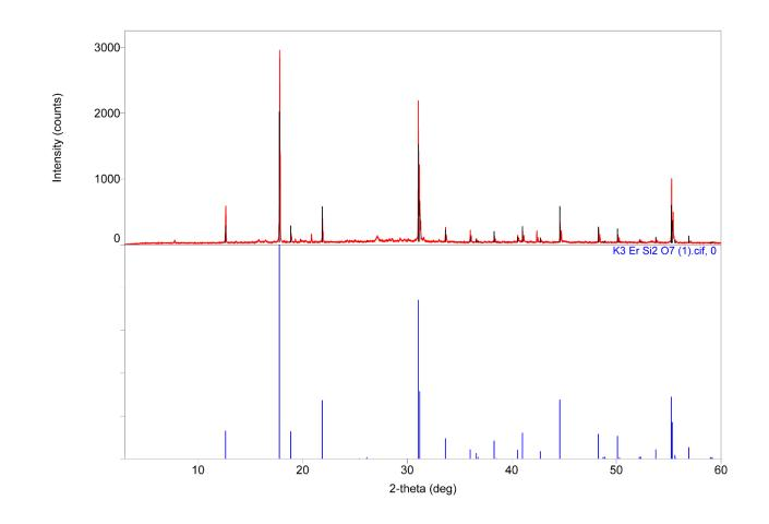
Fig. S1. Powder X-ray diffraction pattern of batch in which crystals of polymorph **1** are obtained. Red pattern represents experimental data, while blue pattern represents overlaid positions of Bragg's peaks calculated from CIF file for polymorph **1**.
