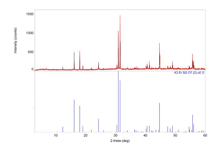
Fig. S2. Powder X-ray diffraction pattern of batch in which crystals of polymorph **2** are obtained. Red pattern represents experimental data, while blue pattern represents overlaid positions of Bragg's peaks calculated from CIF file for polymorph **2**.
