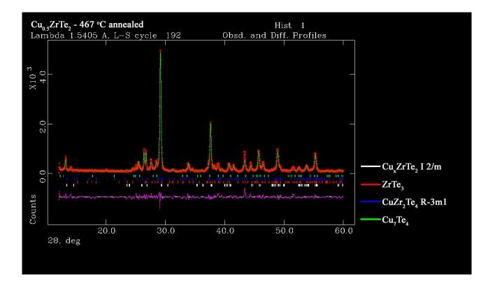
The experimental (green line) and calculated (red cross) X-ray diffraction patterns for Cu0.5ZrTe2 (467 C annealed). As purple line are shown the difference curves between calculated and observed profiles. As colored tick are shown the contributions of the corresponding phases.
