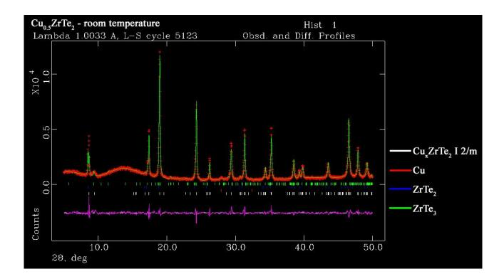
The experimental (green line) and calculated (red cross) X-ray diffraction patterns for Cu0.5ZrTe2 (RT). As purple line are shown the difference curves between calculated and observed profiles. As colored tick are shown the contributions of the corresponding phases.
