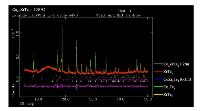
The experimental (green line) and calculated (red cross) X-ray diffraction patterns for Cu0.5ZrTe2 (500 C). As purple line are shown the difference curves between calculated and observed profiles. As colored tick are shown the contributions of the corresponding phases.
