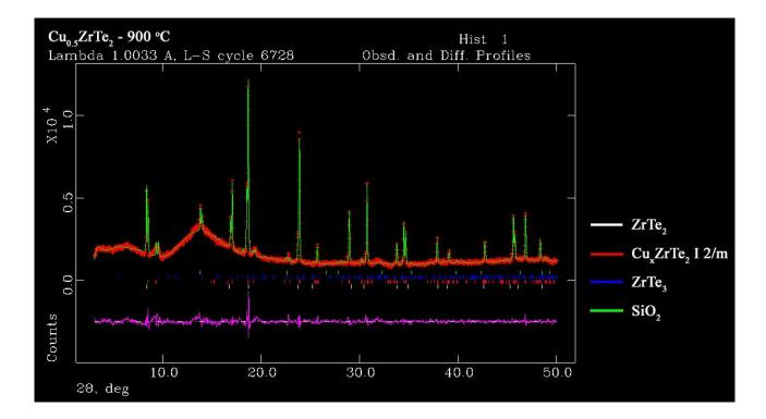
The experimental (green line) and calculated (red cross) X-ray diffraction patterns for Cu0.5ZrTe2 (900 C). As purple line are shown the difference curves between calculated and observed profiles. As colored tick are shown the contributions of the corresponding phases.
