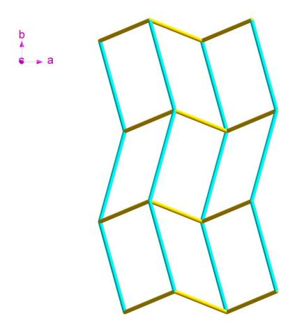
Fig. S3. From a topological point of view, if the Co<sup>II</sup> ions were treated as nodes and the ATBIP<sup>2-</sup> and obix ligands were simplified as linkers, the network can be described as a two-dimensional (4,4) topological network.
