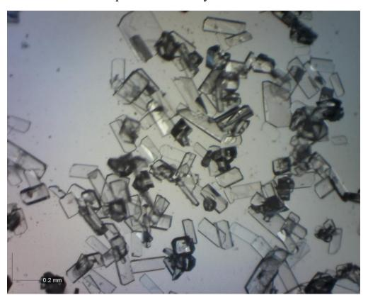
Picture of polymorphs A and B obtained after evaporation to 0.1 of the initial volume of a saturated solution of 2-thiouracil in 0.6 mol dm<sup>-3</sup> HCl
