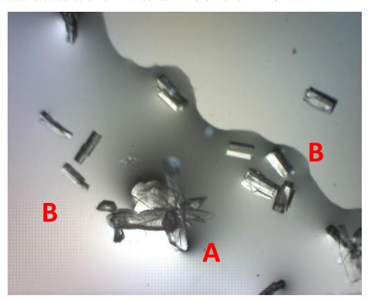
Pictures of polymorph B obtained after evaporation to 0.1 of the initial volume of a saturated solution of 2-thiouracil in 0.8 mol dm<sup>-3</sup> (top) and 1.0 mol dm<sup>-3</sup> HCl (bottom)
