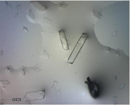
Picture of polymorph A obtained from a saturated solution of 2-thiouracil in 6.0 mol dm<sup>-3</sup> HCl at the begining of crystallization. The solution was saturated at 333 K, filtered and left to stand at room temperature for 2 days.
