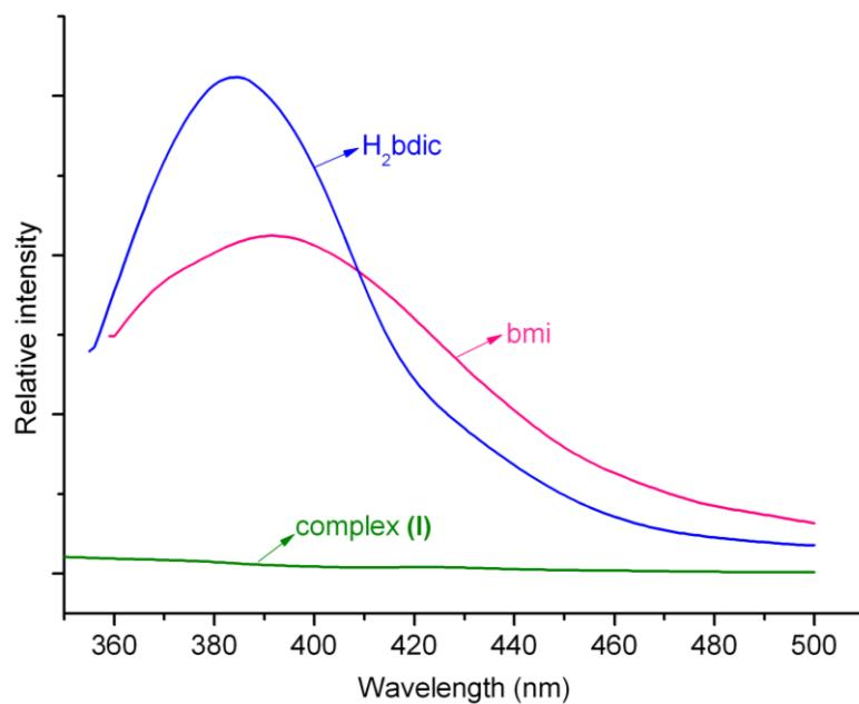
Fig. S1. Solid-state emission spectra of free ligands  $\text{H}_2\text{bdic}$ ,  $\text{bmi}$  and complex (I).
