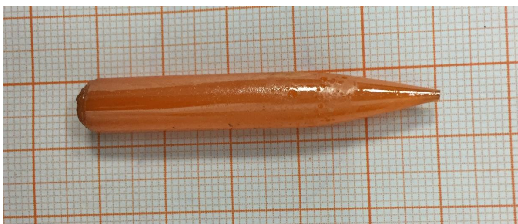
Figure S11. Crystal growth with a growth rate of 0.2 mm/hr.
