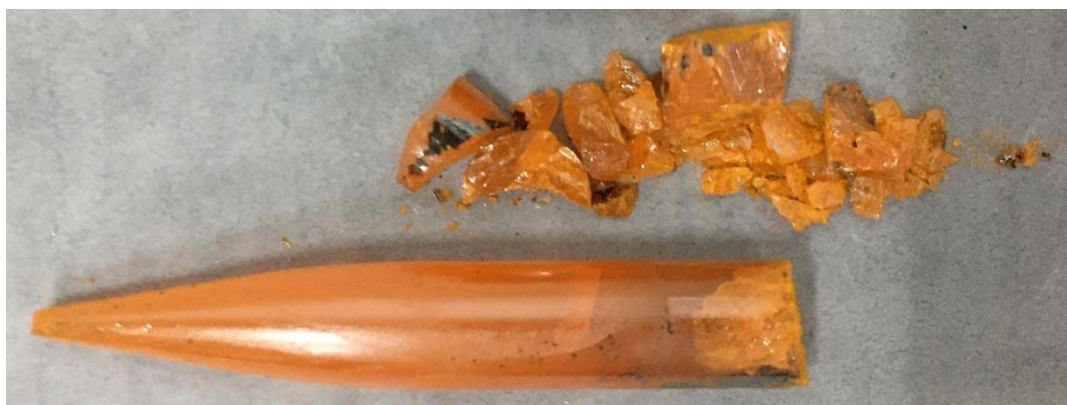
Figure S10. Crystal growth with a growth rate of 1.0 mm/hr.
