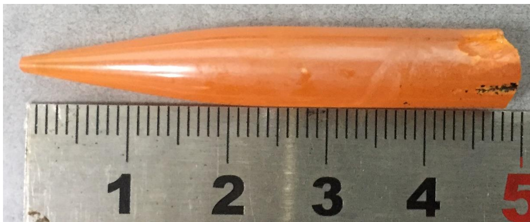
Figure S9. Crystal growth with temperature gradient 8.0°C/cm
