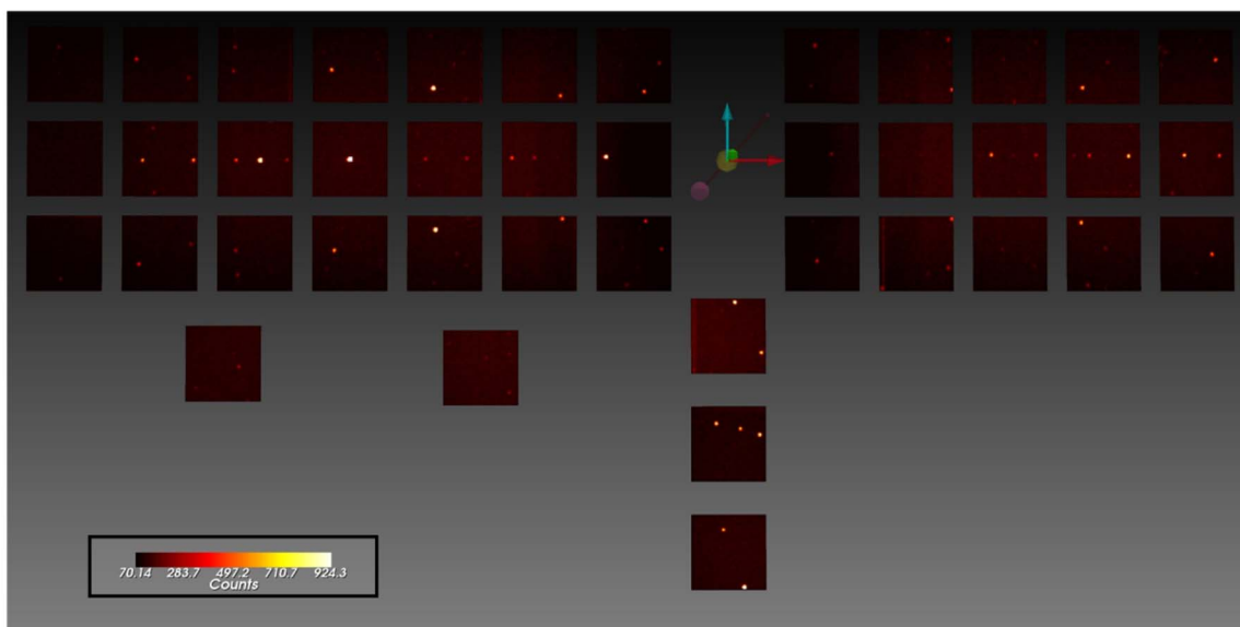
Figure S1 Representative diffraction pattern of NaCl·13D 2 O described by the STARGazer programme (Ohhara et al. , 2009). The diffraction data were collected at 1.7 GPa and 298 K in the diamond anvil cell (Yamashita, Komatsu, Ohhara et al. , 2022) using the Laue-TOF diffractometer at BL18 (SENJU) in MLF J-PARC (Ohhara et al. , 2016). The diamond anvil cell was mounted in the up-side-down orientation ( \chi = 0^\circ ; see Figure 2 in Yamashita, Komatsu, Ohhara et al. , 2022). Diffraction patterns are extracted for time-of-flight = 10–34 ms.
