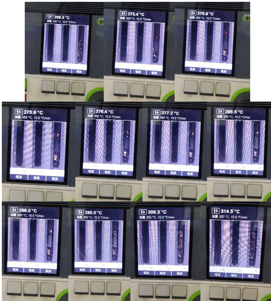
Figure S12 The state of Cis-HNS at 270°C~317°C
