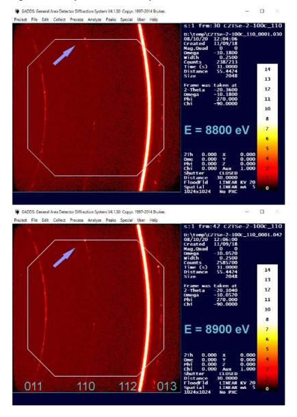
**Figure S1.** A particularly strong spot in the 110 Debye ring of CZTSe is located right at the electronically defined limit of the observation range, which excludes data of lower quality at the edge of the detector.
