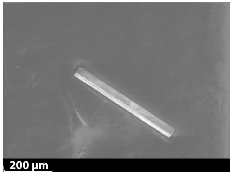
**Figure S1:** SEM image (secondary electrons) of the  $\text{InMo}_4\text{O}_6$  crystal.
