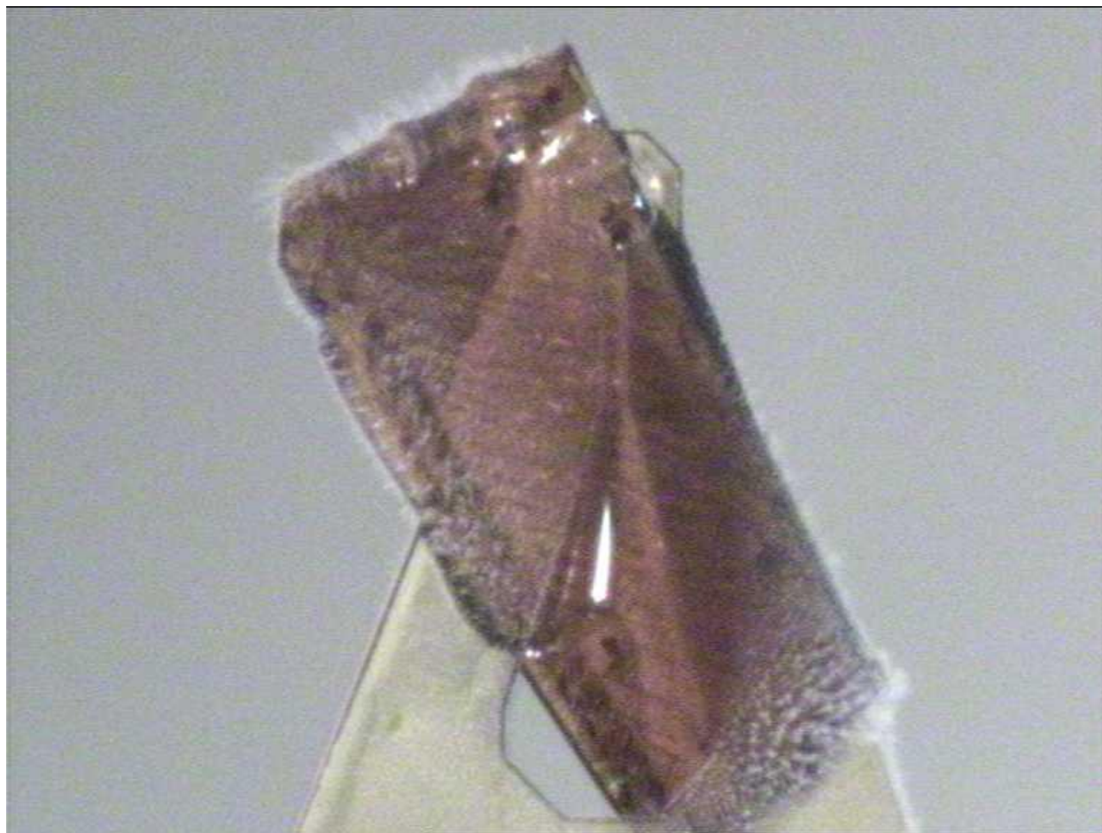
Figure S2 Single crystal of derivative I used in the single crystal X-ray analysis.
