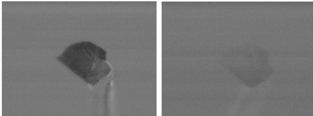
Figure S5 . Microscope photograph of the single crystal of I at the start of the ambient temperature data collection (left) and the 350 K data collection (right) illustrating the similar orientation and morphology of the sample I both \beta - and \alpha -phases.
