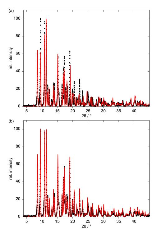
Figure S1 Experimental X-ray powder diagram of clarithromycin (dots) and simulated diagrams (red lines) (a) before optimisation with FIDEL, (b) after optimisation with FIDEL. Experimental data are background corrected.
