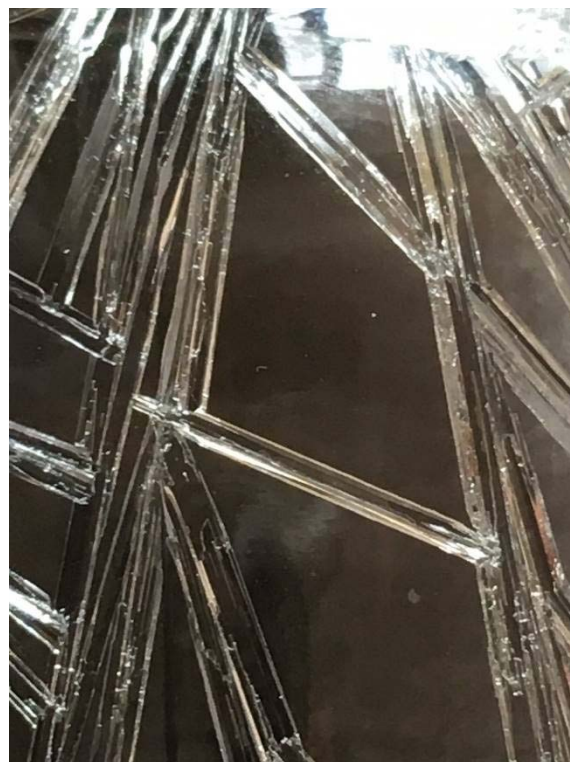
Figure S4 Photographs of the TMP:H 2 O complex showing the rod-like morphology.
