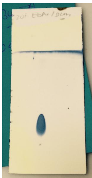
Figure 9. Silica gel TLC plate of Monoolein-d 38 (20% EtOAc in DCM; visualised with Hanessian's TLC stain (ceric ammonium molybdate)).
