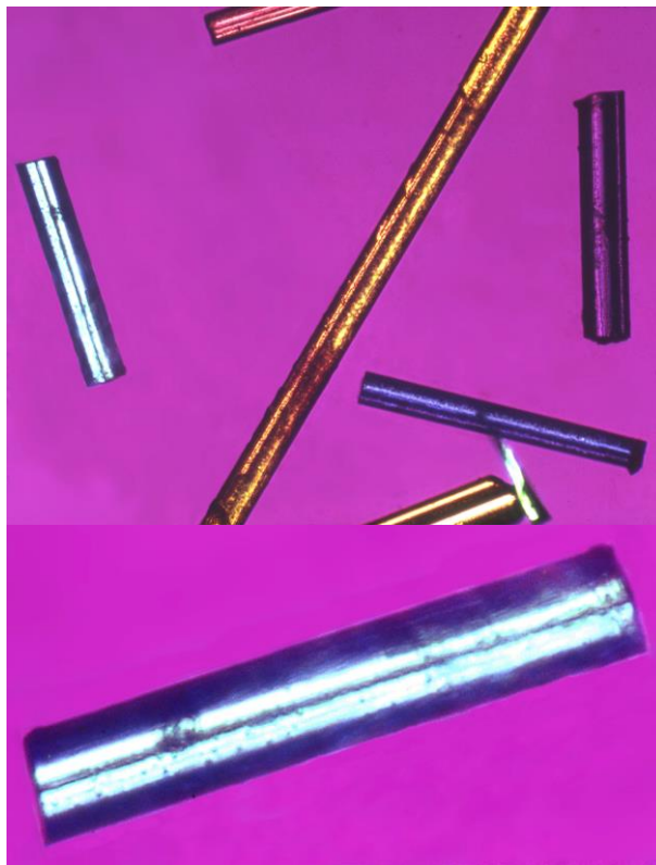
Figure S3.1. Microscopic view of kaliophilite needles from Colle Cimino (crossed polarizers, red I auxiliary plate). The diameter of the magnified needle is about 40 \mu\text{m} . Prismatic faces are clearly visible. In the termination of the hexagonal prisms, basal faces appear to prevail over pyramidal faces.
