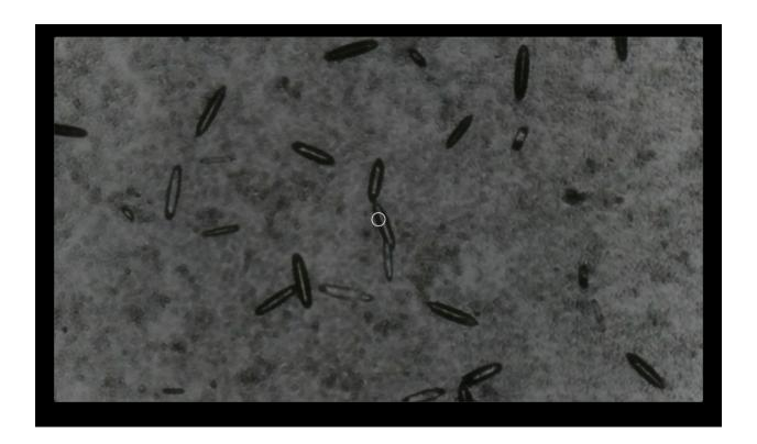
**Movie S2. Simulated data collection for X-ray diffraction.** The targeted Pa497 crystals are translocated into the X-ray beam (white circle of 30 μm in diameter) in a pre-programed sequence according to a crystal ranking. An X-ray pulse is fired at each stop.
