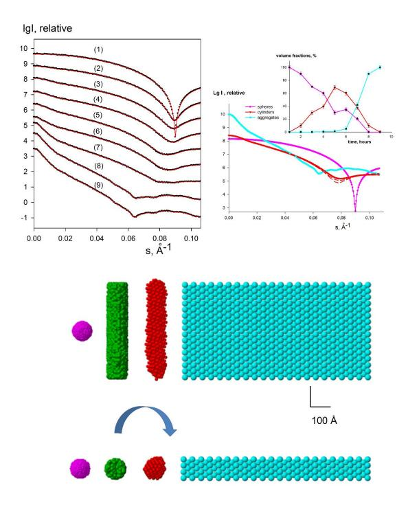
**Figure S1** Simulated scattering curves from an evolving system (initial state, sphere with the diameter 100 Å, intermediate state, cylinder with the diameter 100 Å and height 500 Å, final state – rectangular prism with the side sizes 100, 500 and 1000 Å). The pure species curves from bead
