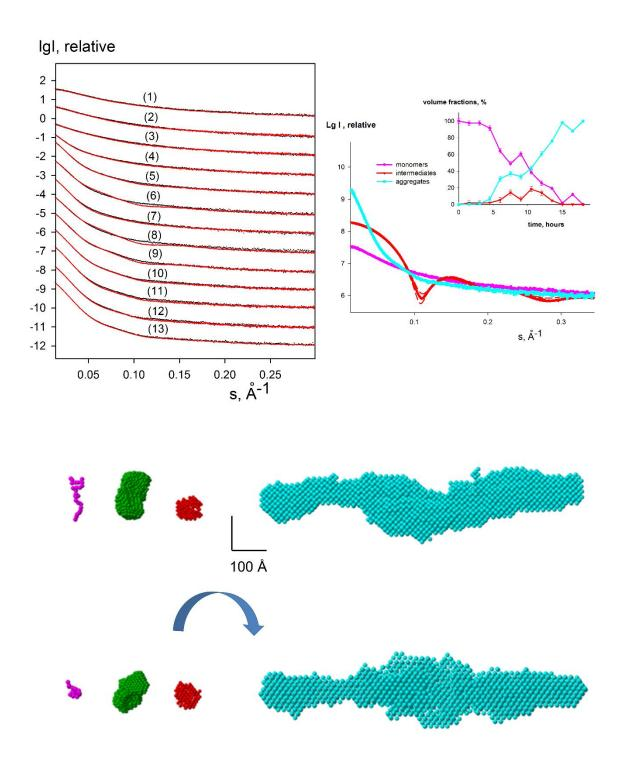
**Figure S2** Analysis of intermediates during  $\alpha$ -synuclein fibrillation. The initial state is represented by a monomer model of  $\alpha$ -synuclein, and the final state by the bead model for the mature fibril (Giehm et al., 2011). Top left panel displays the experimental data (dots with error bars), and the DAMMIX fits as red solid lines. The shapes of the monomer and the aggregates are shown in the
