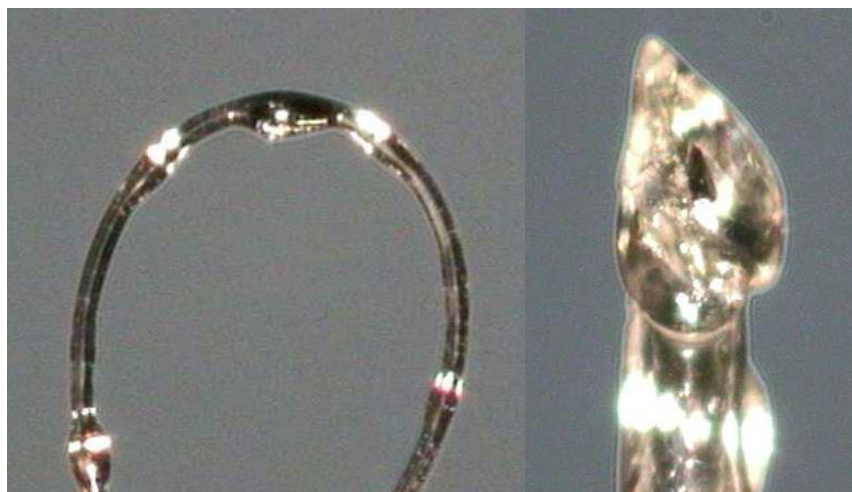
Figure S6 Image of the same crystal mounted on a loop using paratone oil (left), for the LT 100 K and 295 K experiments, and mounted on an amorphous glass rod in Epoxy, two component glue, (right) for the HT experiments.
